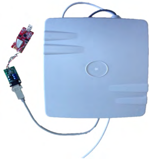
Fig. 2. The RR node embedding the UHF RFID reader.
